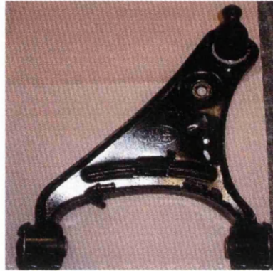
Figure 10.1: Front Upper Control Arm (FUCA)
