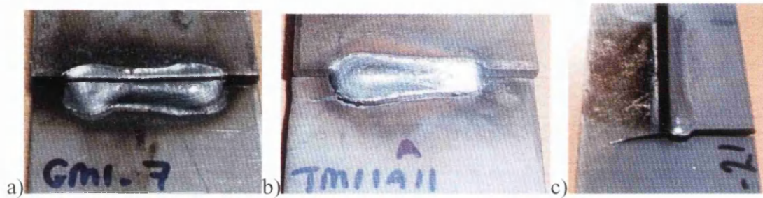
Figure 11.24: Typical Failure Locations for Variable Amplitude SAE Bracket Loading of a) GM1, b) TM11A, c) GM8
